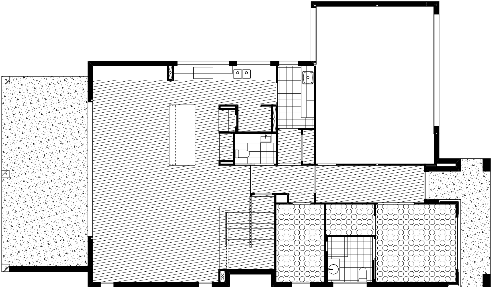
FLOOR COVERINGS (GROUND FLOOR) SCALE: 1:100
